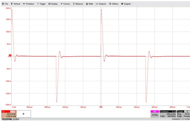
Figure 5: Short circuit with load C \approx 130 \mu\text{F}
